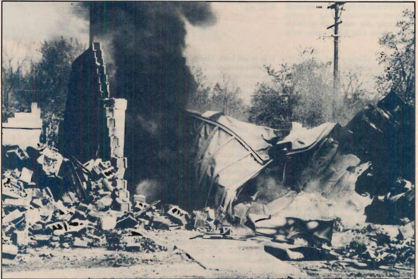
This building was destroyed by lightning which struck a nearby power line sending a surge of electricity to the building's fuse box which burst into flames (Lightning Protection Institute).
